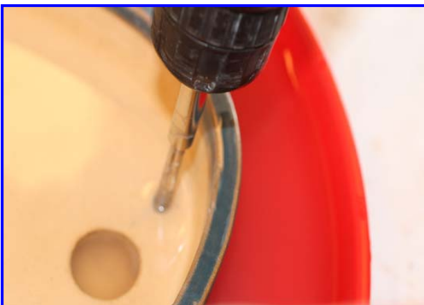
Cordless drill with diamond drill bit attached, drilling wet
